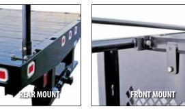
Platform racks are supported in front by the existing cab guard. The rear legs are height adjustable by cutting, with mount brackets that bolt to the platform body frame.
