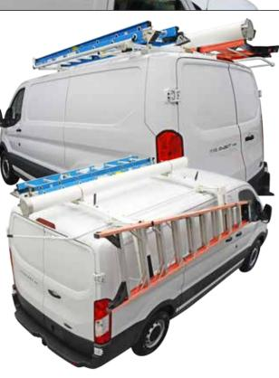
COMBO RACKS WITH BOTH EZ LO-DOWN AND CLAMP & LOCK UNITS ARE AVAILABLE FOR LOW ROOF AND COMPACT VANS.
